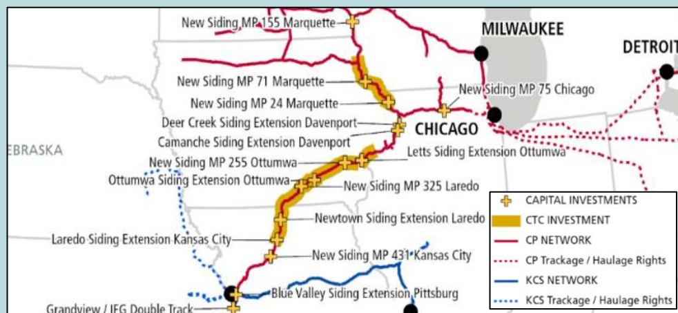
Figure 25: Railroad Improvements Planned Along the CPKC Lines
